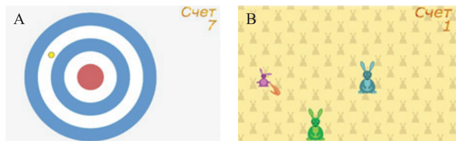
Fig. 1. Stability training: A - static test "Target", the patient, by shifting the center of the pressure, needs to move the yellow dot to the center of the target and hold it in this position for the maximum amount of time (until the end of the test series); B - dynamic test "Hares", the patient needs to move his hand by shifting the center of the pressure to capture the hares
